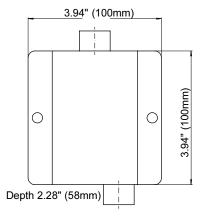
Cable junction box Part# 2074460 The cable junction box is rated NEMA 3S / IP 54 and is suitable for mounting outside tanks or shafts or inside dry control boxes.
