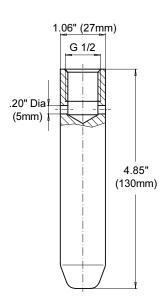
Additional weight Part# 1524399 The additional weight replaces the protective cap and helps to stabilize the transmitter in turbulent conditions. Weight: approximately 1.1 lb, 316ss.
